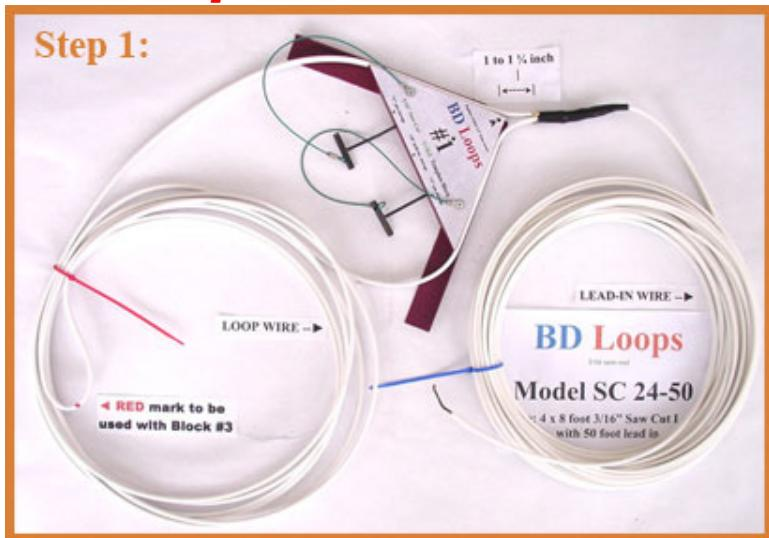
Place saw-cut yoke (where the loop meets the lead-in) into the #1 block red side down with a 1 to 1 $\frac{1}{4}$  inch space from top of block to split of yoke.
