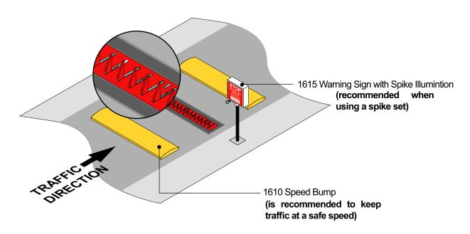
To lower or raise the spring loaded spikes, slide the bars through the small slots and lock on to the spike rod.
