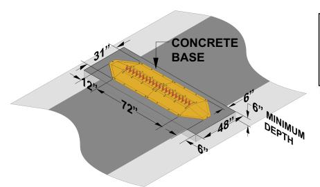
Spikes must be anchored to a concrete surface. If you do not have a concrete surface (see Safety First on page 4), you will need to create a concrete base before installing the surface spikes (refer to illustration for suggested minimum dimensions for concrete base).
