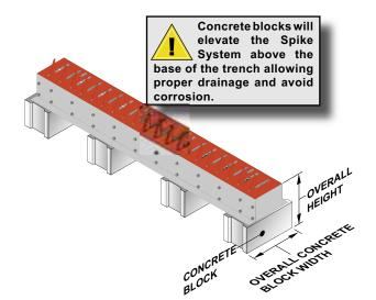
Dig a trench using to the overall height and concrete block width (see dimensions above).
