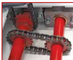
transfer box provides direct mechanical linkage
